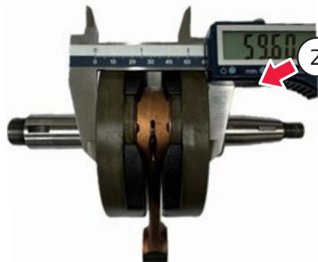
Connecting rod tolerance
