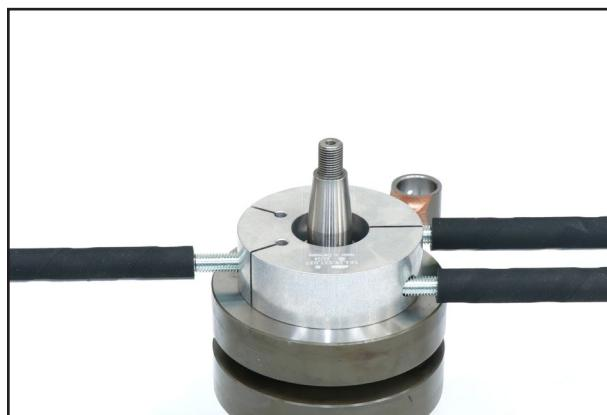
**Disassembly of the water pump**
