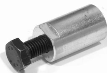
This tool is used to secure various sprockets and to loosen or tighten engine nuts and bolts.
