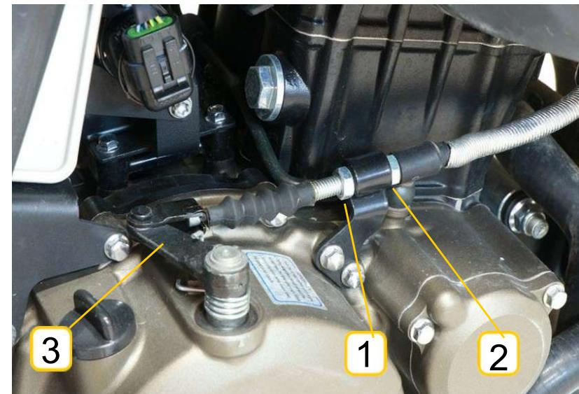
After the adjustment, start the engine and check the clutch operation. If the clutch slips or it is difficult to engage a gear, readjust it.
