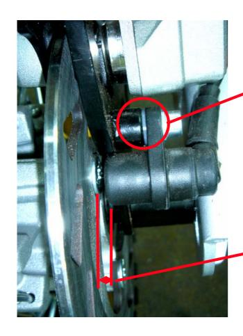
Plastic washer needed to assure the correct distance.
