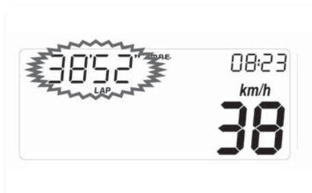
The chronometer is set in operation automatically with the first pulse from the speed sensor and stops 3 seconds after receiving the last pulse from this sensor.
