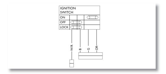
Use a meter to check that there is a circuit between the ignition switch connector cables.
