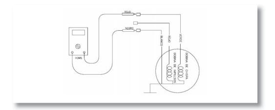
Spark condenser charging coil resistance.
