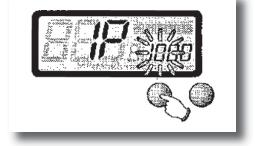
Press the selection button 3 times to change to adjustment of the sensor points.
