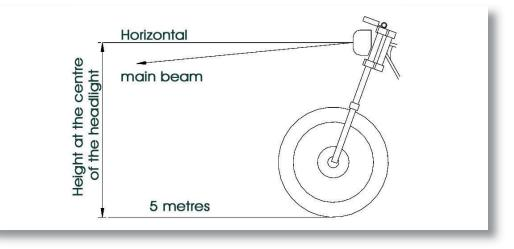
With the rider seated on the machines, the headlight beam should be adjusted in such a way that the main beam is situated below the headlight horizontal.
