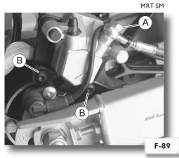
MRT Unscrew the connector using the bolt (A/F-90).
