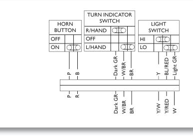
Check that there is a circuit between the connector cables.
