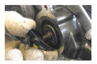
• Unscrew and remove the oil filter plug.
