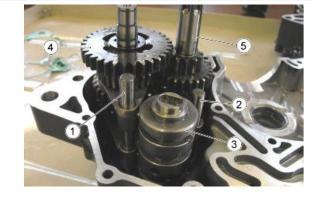
• Apply oil for gears on the grooves of the desmodromic drum.
