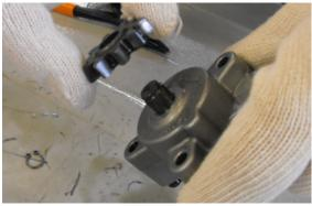
• Remove the pump gear.
