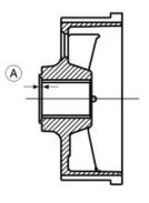
Check the clutch hub for damage and wear that may result in clutch irregular operation. If necessary, replace the hub.
