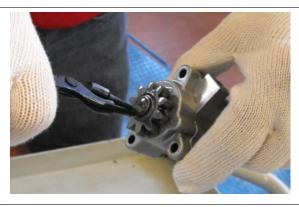
• Remove the pump gear.
