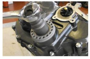
• Remove the spring and oil filter.
