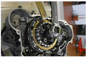
• Remove the shim and the clutch housing.
