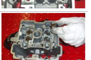
• Compress the valve spring using the tool.
